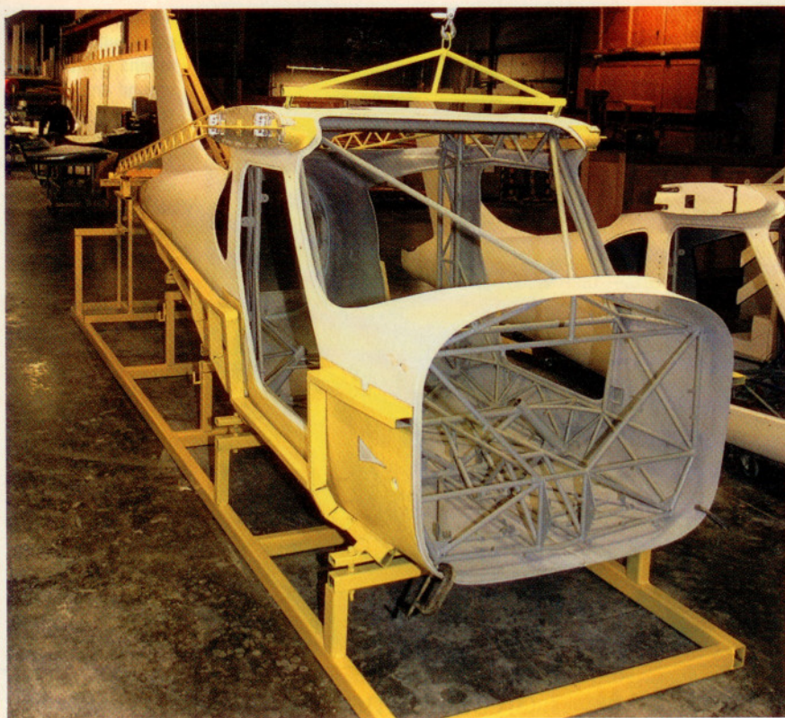
The Lycoming kit engine resides in a thousand parts at Barrett Precision Engines (opposite page, left). The Customer Assembly Center at Glasair Aviation (opposite page, right) is equipped with special tools and fixtures that would cost thousands of dollars for a homebuilder to reproduce. The "yellow monster" is a new fixture that helps locate the steel-tube cage inside the composite fuselage shell with great accuracy (left). Monty Barrett, at home in the engine test cell control room (above).
